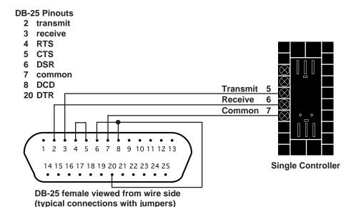
Figure 2.2 -EIA-232 Interface Wiring Diagrams.
