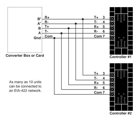
Figure 2.4 -EIA-422 Interface Wiring Diagrams.
