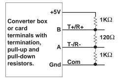
If the system does not work properly it may need termination resistors at each end of the network. A typical installation would require a 120-ohm resistor across the transmit/receive terminals (3 and 4) of the last controller in the network and the converter box or serial card. Pull-up and pull-down resistors may be needed to maintain the correct voltage during the idle state.
