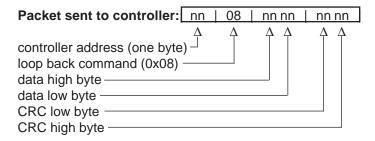
Example: Run loop back test on controller at address 40 (0x28).
