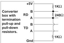
If the system does not work properly it may need termination resistors across the receive A and B terminals at the converter. A typical value would be  $240\Omega.$  Pull-up and pull-down resistors may be needed to maintain the correct voltage during the idle state.
