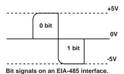
Figure 1.3 - Interface bit signals.
