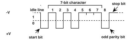
Figure 1.5 - ASCII upper case "W" with start and stop bits.
