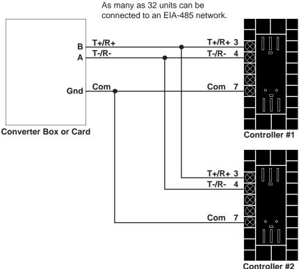
Figure 2.3 -EIA-485 Interface Wiring Diagrams.
