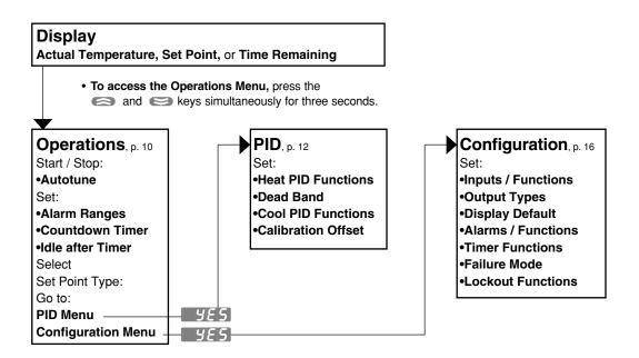
At the Pid or [nF9] prompt, press and hold the SED key, and the or key to select yE5. Release the keys to move to the new menu.
