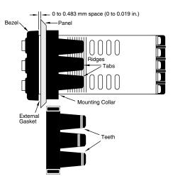
Figure 13- Case Rear View and IP65/NEMA 4X Seal Example
