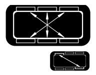
NOTE: To guarantee a proper IP65/NEMA 4X seal, make sure the gasket between the panel and the rim of the case is not twisted and is seated properly. Press firmly.
