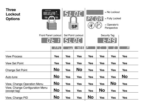
Note: Front Panel Lockout requires an external hardware switch. For set-up and wiring information, see p. 23. For more wiring information, see p. 43.
